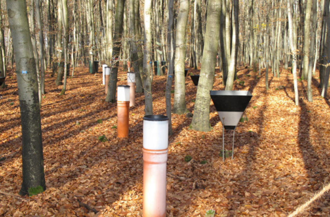
Experimental site: measurement of precipitation (© ForeStClim)
