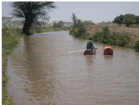
b. Canal profile surveying
