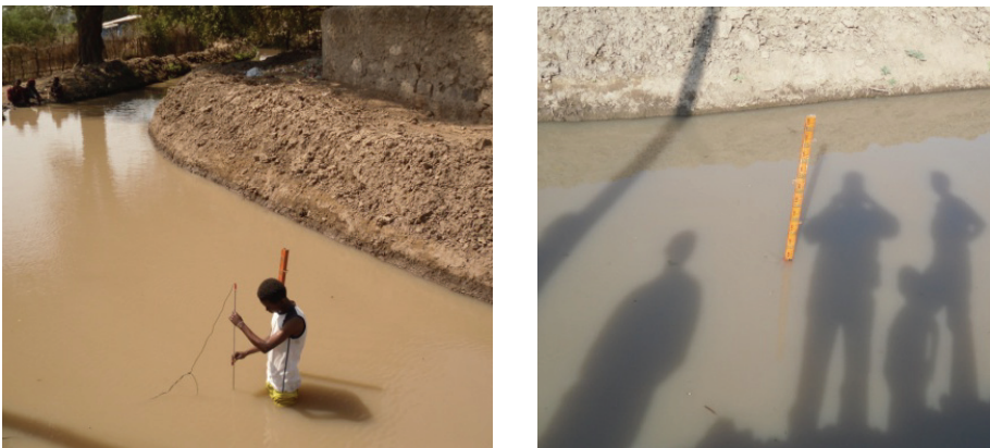
Figure G.1. a. Current metering, b. Flow depth measurement at a control section, for stage-discharge relation at Golgota Scheme
