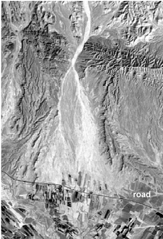
Figure 13-10 Alluvial fan with large active part where most of runoff is lost by transmission loss, except runoff of largest floods. Note absence of drainage lines south of road. TM, band 5. Central Iran. Distance EW is 8.5 km.
