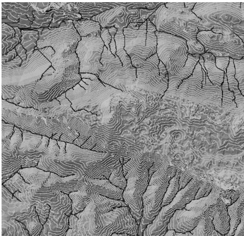
Figure 3-2 DEM created from stereo aerial photographs, with visualization by way of contours and hill shading and automated determination of drainage lines. Note sinkholes in karst area at high elevation area in the central part of the image. Source: Maathuis (unpubl.).
