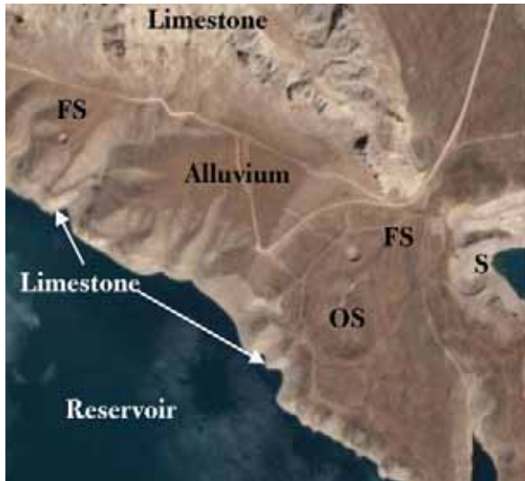
Figure 9-6 Collapse sinkholes in river terrace deposits, near a reservoir in north Iran. Freshness of features indicates relative age: FS recent; S older; OS oldest collapses. Reservoir suffers from loss of water through karst conduits. High-resolution satellite image. Distance E-W is 1.3 km. Source: Google Earth
