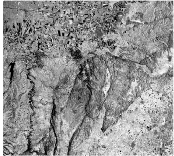
Figure 5-12b TM thermal band (b 6), resampled to same pixel size as fig.5-12a. Note relief features associated with faults/fractures.
