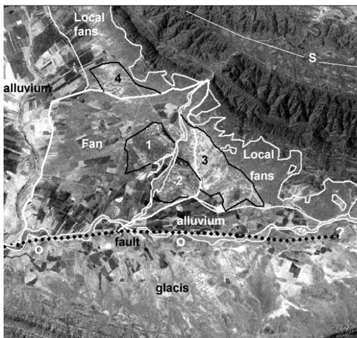
Figure 13-20 Subsidence area bordered in south by a fault, note outcrops (O) and in the north by the flank of syncline (S), axis shown. Thickness of fanglomerates in central part of subsidence area is >100m. Alluvial cover is shallow south of the fault (glacis) and in the area with local fans. 1 = oldest canal-overflow basin type of flood-spreading scheme, scheme 2 is more recent, scheme 3 is under construction, while scheme 4 makes use of local runoff. Flash flows from the river draining the syncline are diverted. River is unstable between schemes no's 1 and 2. Irrigated agriculture benefits from groundwater recharge. Gareh Bygan area south-central Iran. TM band 8 (14.25 m resolution). Distance EW=14.8 km.
