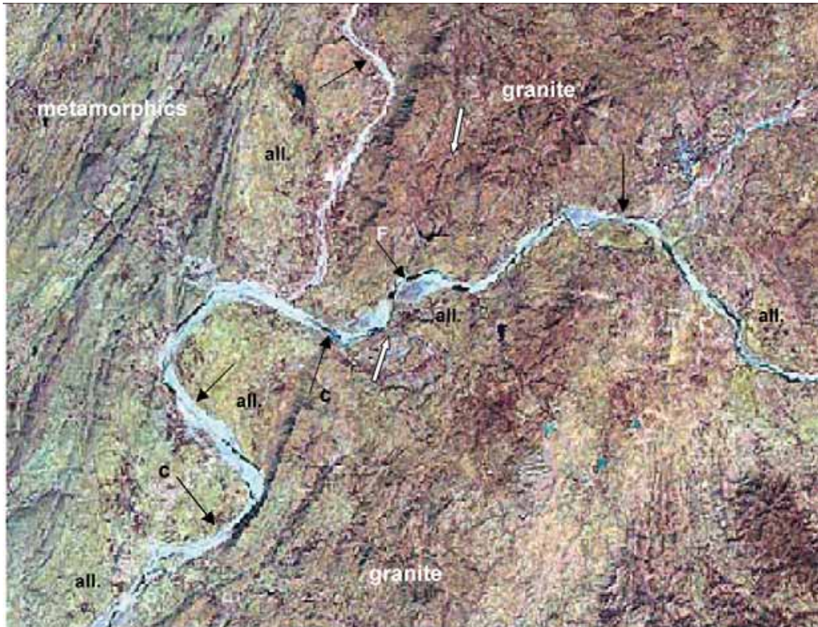
Figure 13-2 Dhamni River in north Gujarat, India, with possible recharge sites for weirs or sand dams (black arrows). All. = alluvium, (c) = contact zone metamorphics and granites. White arrow indicates site on lineament (fracture, F). Sites and alternatives need to be checked in the field. Distance E-W is 14 km. Landsat ETM+ image
