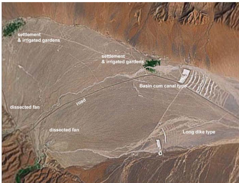
Figure 13-21 Alluvial fans SE of Yazd, central Iran, showing two types of recharge schemes on the non-dissected part of the alluvial fans. Schemes were constructed to augment groundwater, which is brought to Yazd city (not shown) by means of long qanats. Clay accumulation (30 to 40 cm) in the Basin cum canal type of scheme proved to be impermeable. The coarse-grained deposits in the long dike type of scheme were more permeable during test period but had significant evaporation loss. Image shows the difficulty of positioning and designing intakes because of flash flows. The dissected part of the upper fan is not suitable because infiltration-overflow canals along contours will be very sinuous. Source: Google Earth
