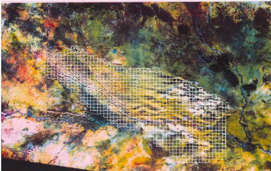
Figure 11-2 Numerical model grid build over the integrated image of Landsat TM false colour composite (bands 4, 7, 1) with the second vertical derivative of the aeromagnetic total field intensity (Lubczynski et al., 1996). Grid cells with triangles represent northern inflow.
