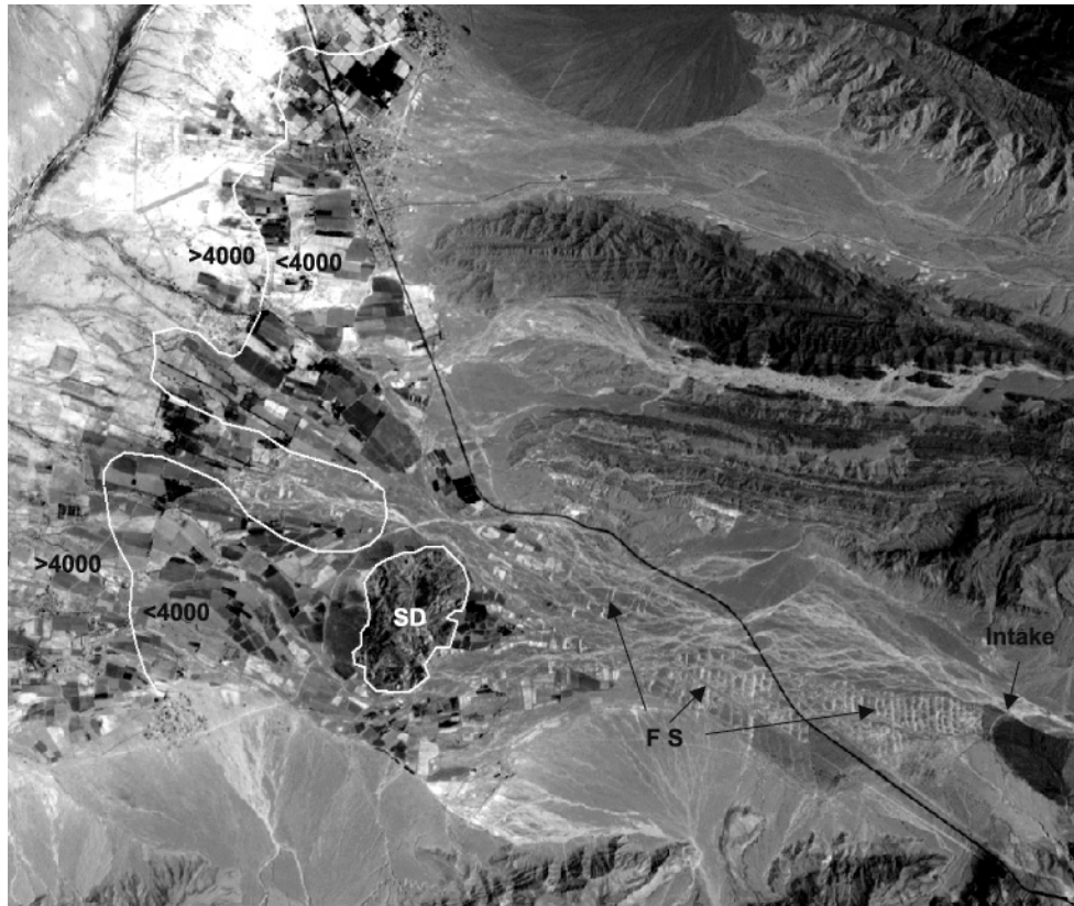
Figure 13-15 Alluvial aquifer of Sarchahan Plain, salt dome (SD) and flood-spreading scheme (FS), south Iran. West of white line, electrical conductivity of groundwater is > 4,000 \mu\text{S} , east of line EC is less. Agricultural area (irrigated by groundwater) coincides roughly with \text{EC} < 4,000 \mu\text{S} , while the salt dome has minor influence on groundwater quality distribution. Landsat ETM
