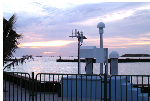
Figure 4. GLOSS Core Network tide gauge station No. 28 at Male, Maldives equipped with a continuous GPS receiver (high-st dome) collocated with water level sensors (photo courtesy of D. Caccamise).
