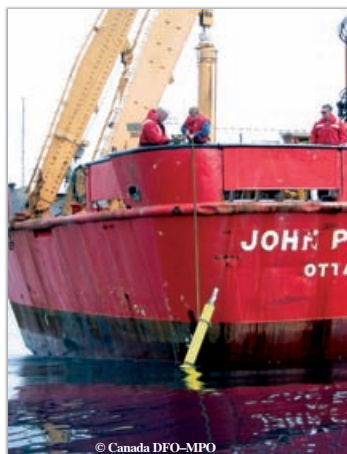
© Canada DFO-MPO An Argo profiling float being deployed from the Canadian coast guard ship John P. Tully in the Gulf of Alaska
