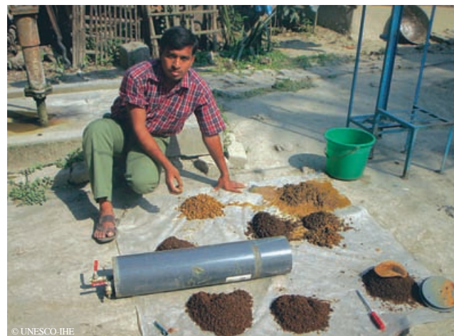
Inspection of a family filter after one year of continuous operation. The used iron oxide-coated sand is a dark brown colour. Iron oxide is commonly known as rust
