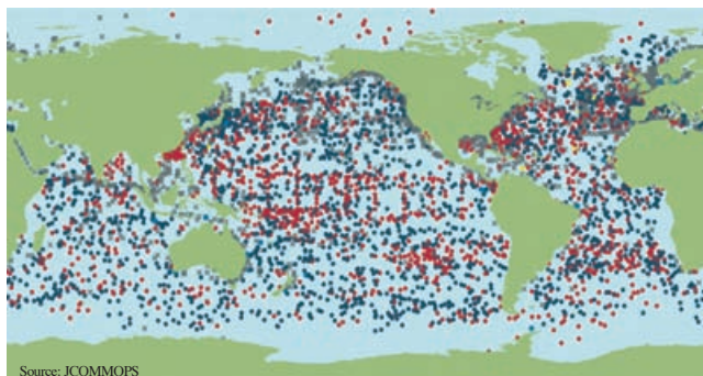
Source: JCOMMOPS Towards global coverage: in situ platforms observing the ocean in October 2005, which produce data available in real time. These data come mainly from Argo floats (dark blue), ships of opportunity (light grey, light blue and yellow), fixed moorings and drifting buoys (red). The seasonally ice-covered oceans pose technical problems that are yet to be surmounted
