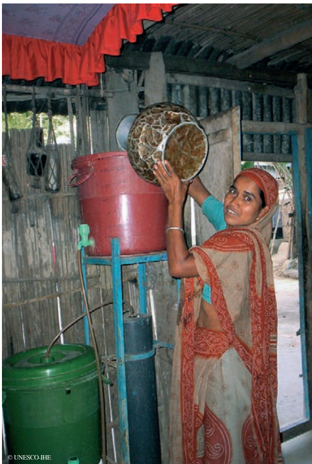
In the five-member Hassan household in Bhabanjpur (Raibarij), Mrs Hassan is pouring water into the family filter to remove any arsenic the water may contain. The filtered drinking or cooking water will be collected in the green container beneath the filter
