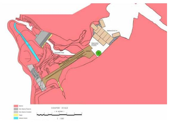
Updated site plan showing the exposed bedrock below the western dam and at the eastern cliff. The drawing also shows the extended ranges of gabions at the eastern inlet of Wadi Al Jarra into the retention basin of dam nr. 3. The plan reproduced here is not to scale.
