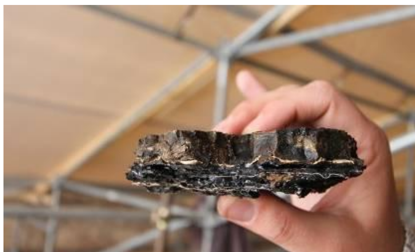
Figure 111: thickness of the bitumen layer changing from 2-3 cm on the top of the roof to 4-5 cm at the lower levels
