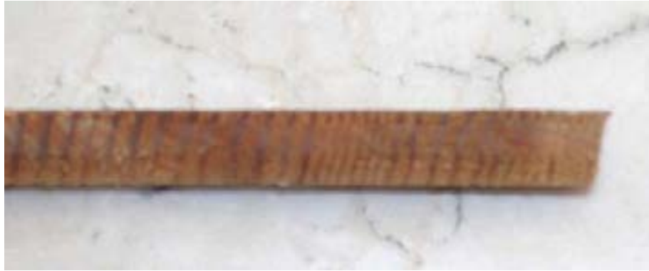
Figure 33: the sapwood limit on the sample AN07SaeS.
