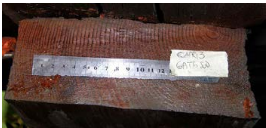
Figure 27: a digital image of tree-rings in the truss 3.
