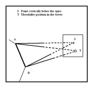
Figure 4. Principle of offset measurements.
