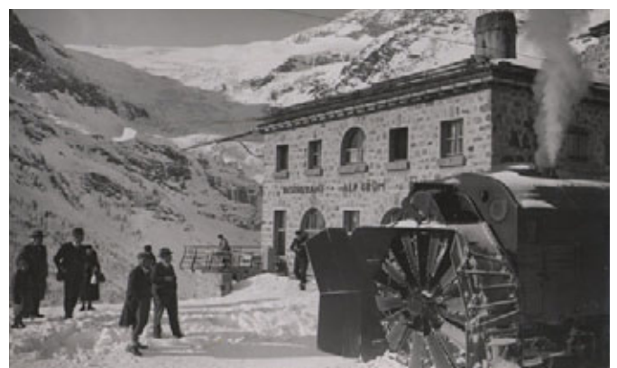
Bernina line > The R 1051 steam snow blower, built in 1911, in front of the Alp Grüm reception building. Rhaetian Railway
