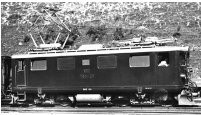
Bo'Bo' > After 1947, passenger trains were hauled by the Bo'Bo' locomotives, permitting higher speeds. Collection G. Brüniger
