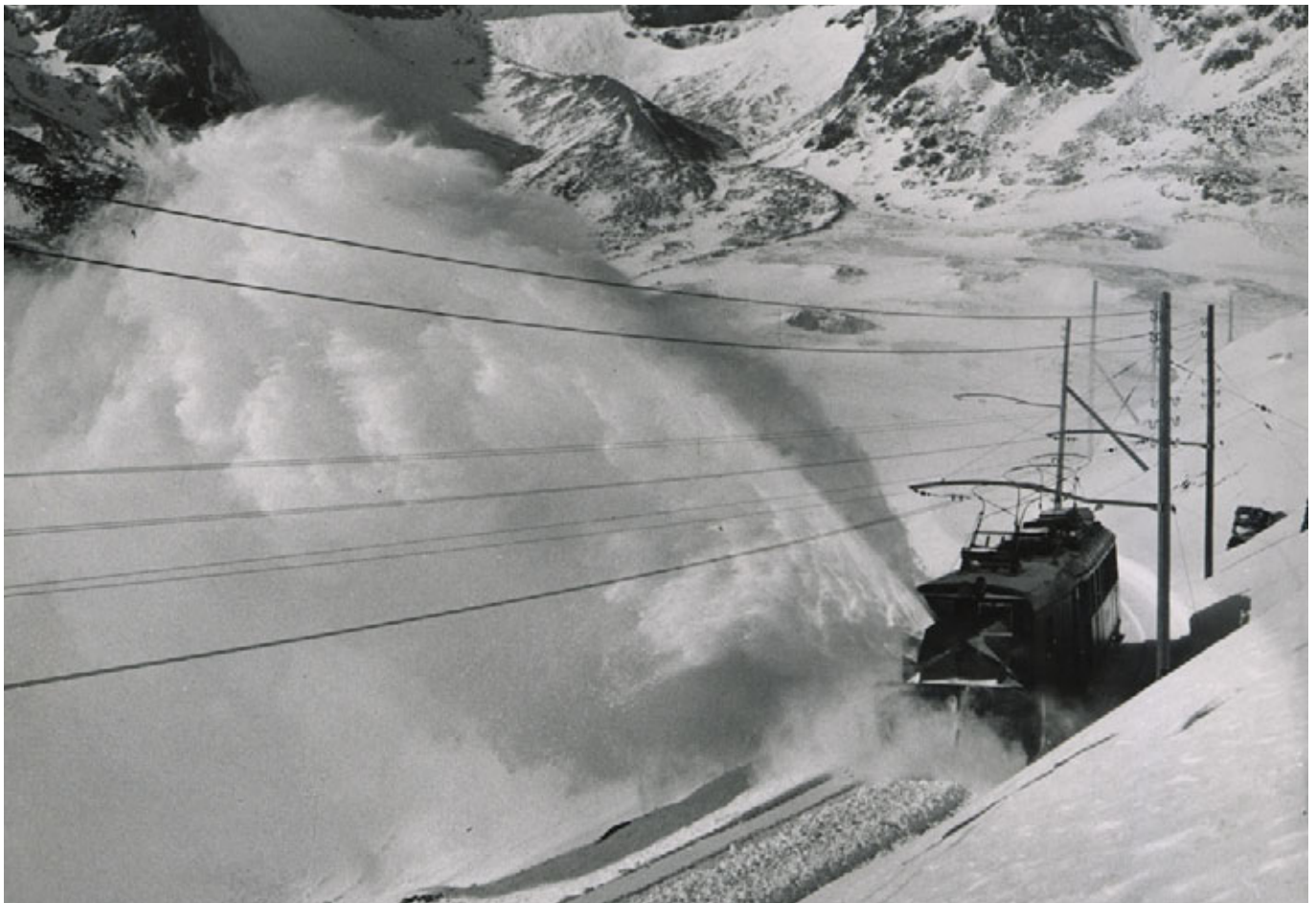
Bernina line > The first Rhaetian Railway electric snow blower: 1943. Here it is in operation between Arlas and Ospizio Bernina. Rhaetian Railway
