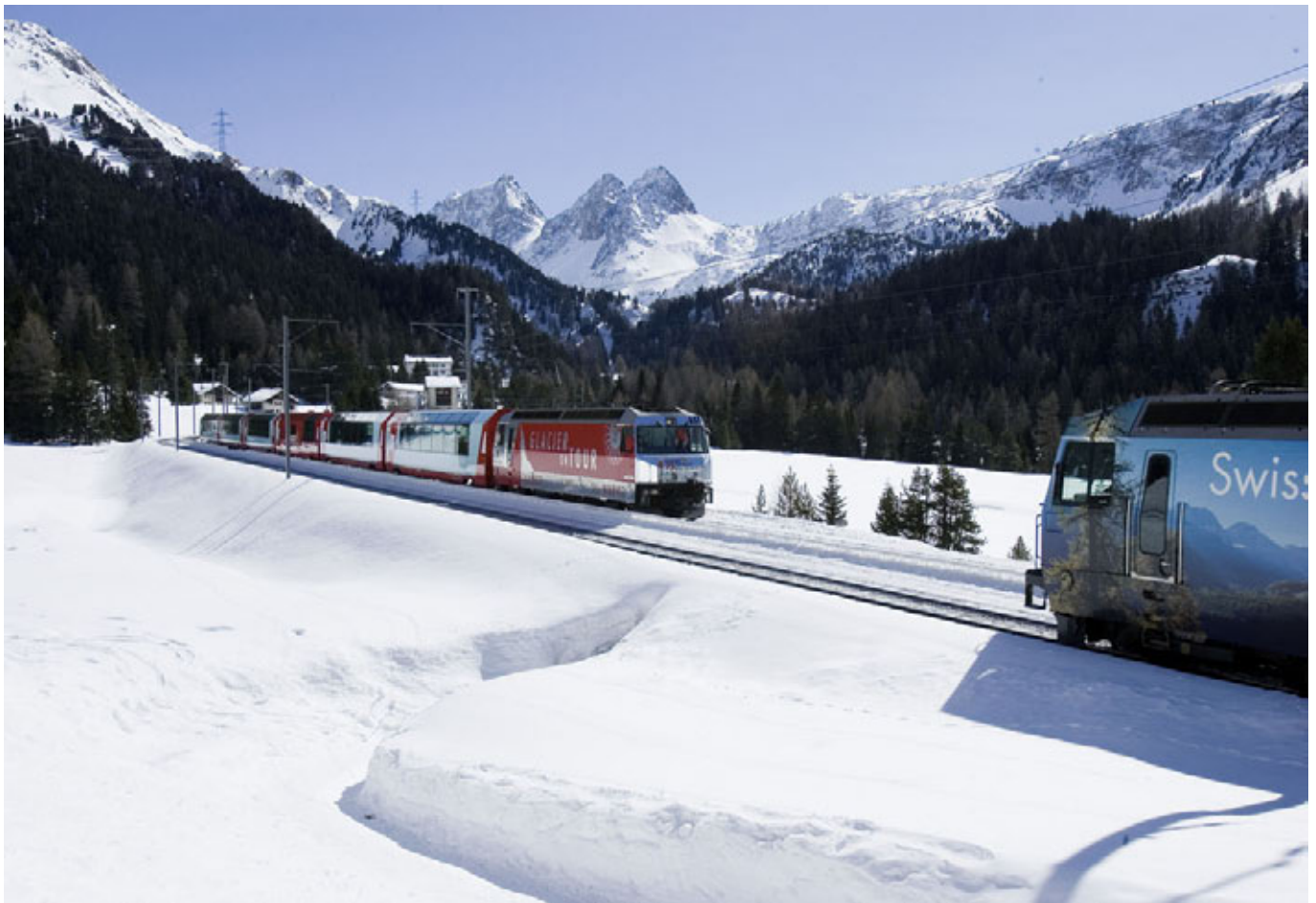
Preda > Extended stretches of double track, like here in Preda, make it possible for trains to cross without stopping. A. Badrutt
