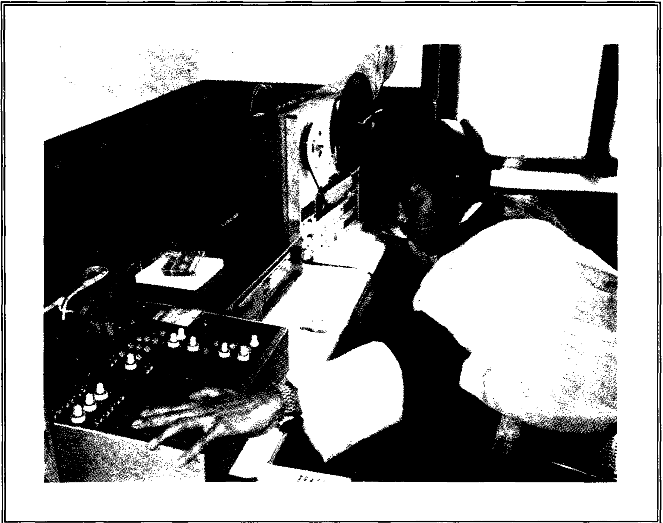
BBS technician mixes tape inputs on the temporary editing console installed at BBS (Photo UNESCO/CAA 1991).
