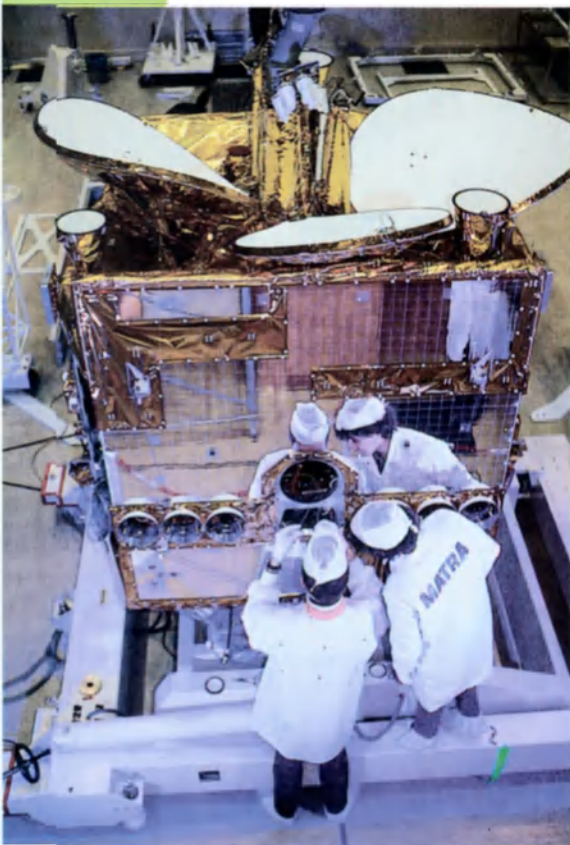
The SPOT-1 satellite under construction in Toulouse (France) in 1984. This family of earth-observation satellites provides black and white photos of the earth within an accuracy of about 10 metres and reconstitutes relief.
