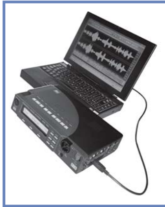
A recorder connected to a portable digital editing console for the transfer of recorded material. The transferred audio will then be edited during post production.
