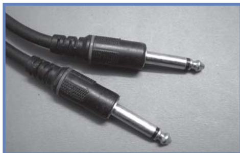
A pair of ¼" phono jacks. Both are mono connectors, as indicated by the single black band.
