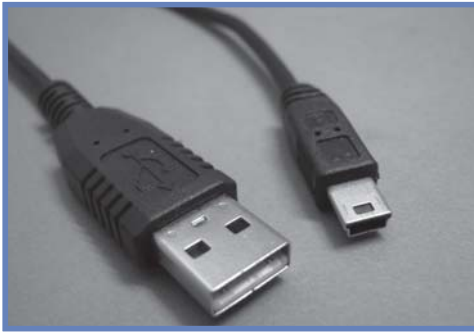
Regular size and mini-USB connectors, both male
