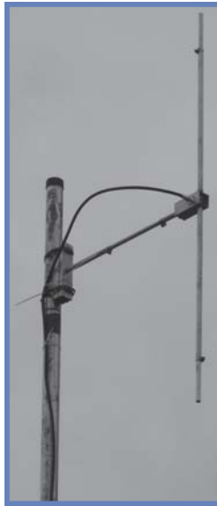
A simple homemade dipole antenna. This unit is mounted on a large bore metal post.
