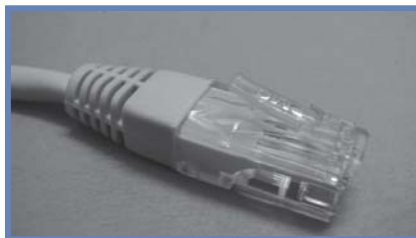
An RJ-45 LAN connector. The 8 wires of the LAN cable need to be crimped in place.
