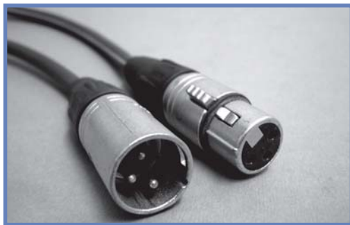
A male and a female XLR connector. Note the tab on top that must be pressed to disconnect the connector.
