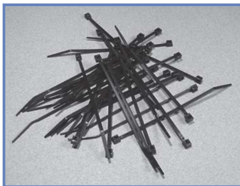
A selection of cable ties. The tip is looped around the cables that need to be tied together and through the box at the other end of the tie, which locks the loop in place
