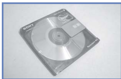
A standard MD disc. The shutter moves aside during recording to let the recorder access the actual disc surface.
