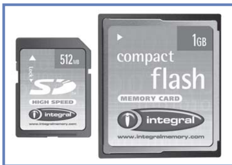
Secure Digital (SD) and Compact Flash (CF) memory are solid state and have no moving parts. Very small cards can now give several hours of broadcast quality recording.
