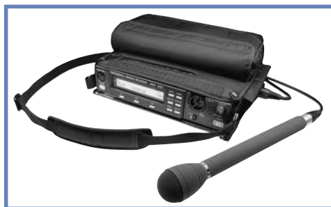
A basic digital audio recording kit. Note the case within which the recorder is carried to protect it from dust.
