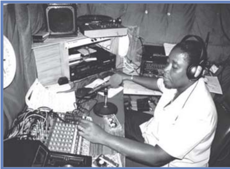
A studio in Radio Toco, Trinidad & Tobago (Caribbean). This one uses cloth and padding for the walls.
