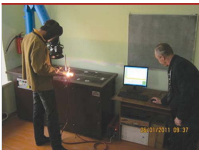
Gas Welding Training on Computer Simulator. RIPO Branch "Industrial Pedagogical College." © RIPO
