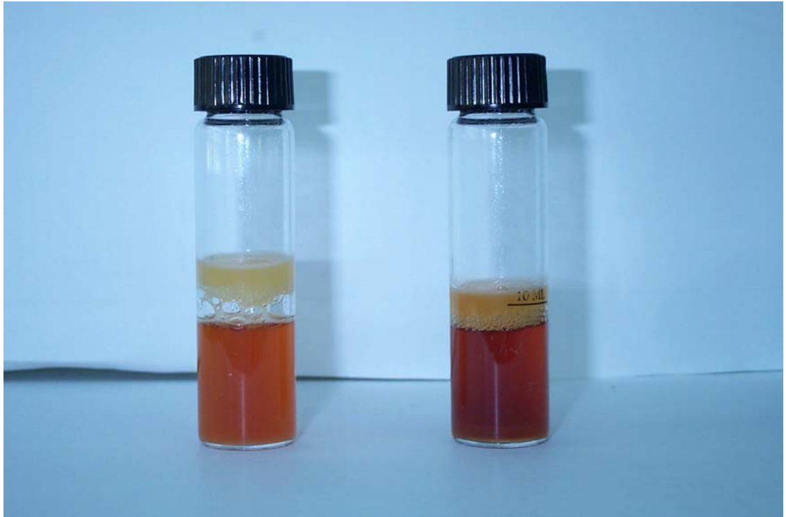
Test showing the presence of Coli form Bacteria in water sample
