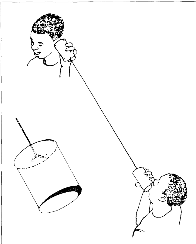
6. Make your own telephone from two tins and a 6 metres length of string. Pull the string tight while you talk. [Page 8.]
