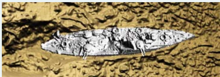
Digital image of Danton obtained from multibeam side scan sonar data. Galsi/Fulgro contract.
