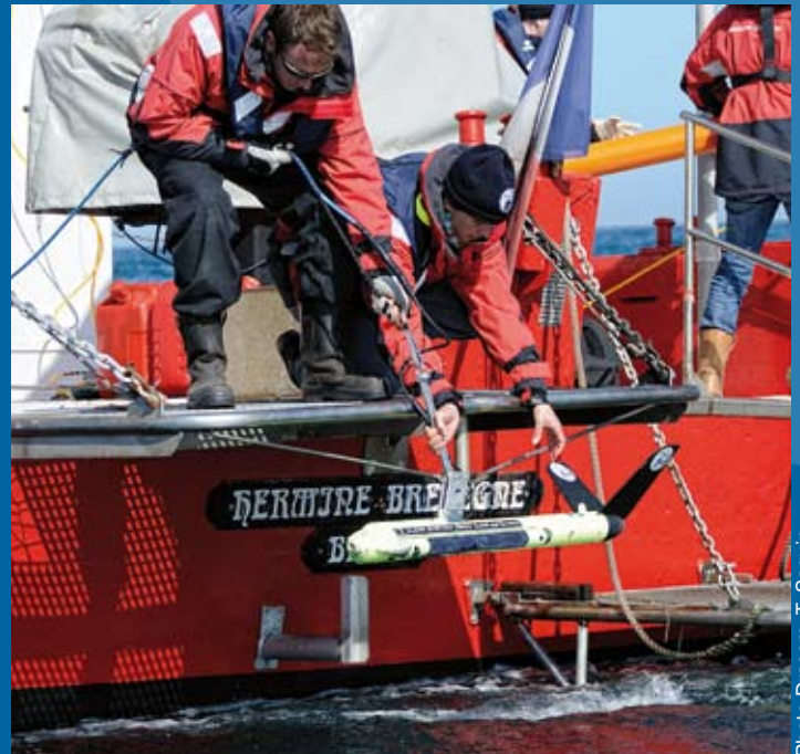
Lowering the side scan sonar fish into the water. European project of the Atlas of the Two Seas.
