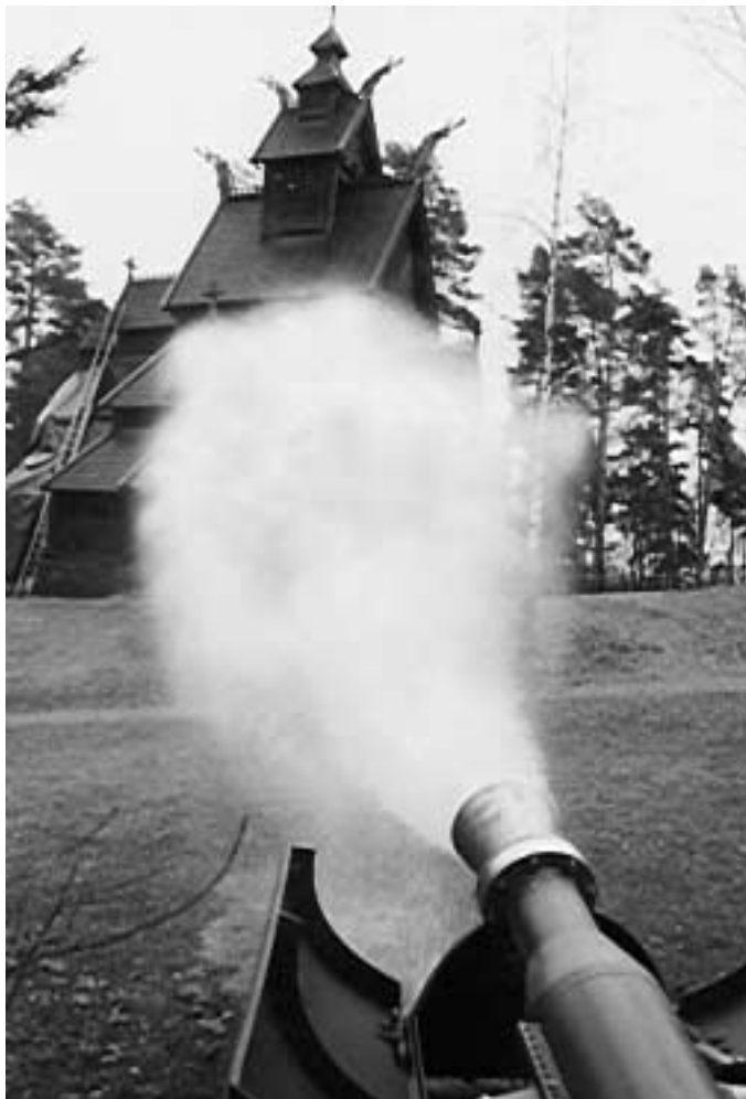
Testing a unique water cannon (water-mist fire extinguisher) Photo: author
