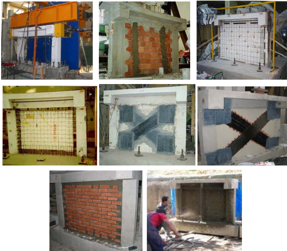
Figure 3. A number of tests on one bay-one story reinforced concrete infilled frames
