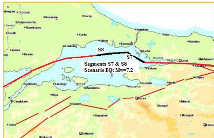
Figure 3. Considered scenario earthquake along the fault segments S7 & S8 in Marmara Sea
