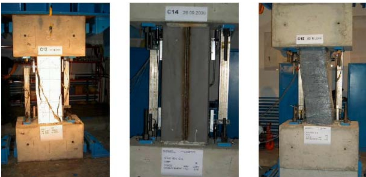
Figure 6. Test on RC columns (original specimen, retrofitted specimen with steel plate and with CF sheet)
