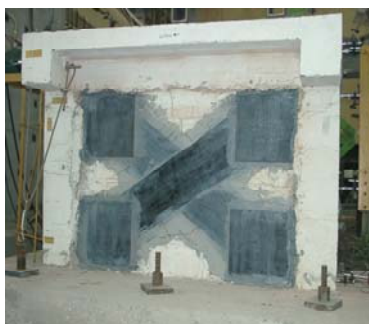
a) Integrated infill frame with pasted CFRP before testing
