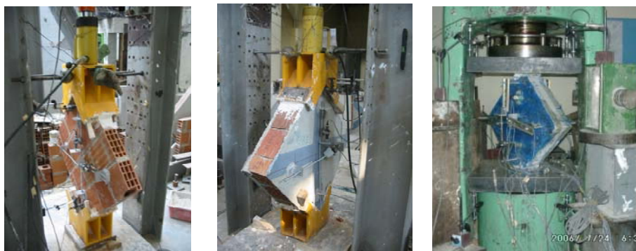
Figure 2. Diagonal tension (pure shear) tests on the original and the retrofitted specimens
