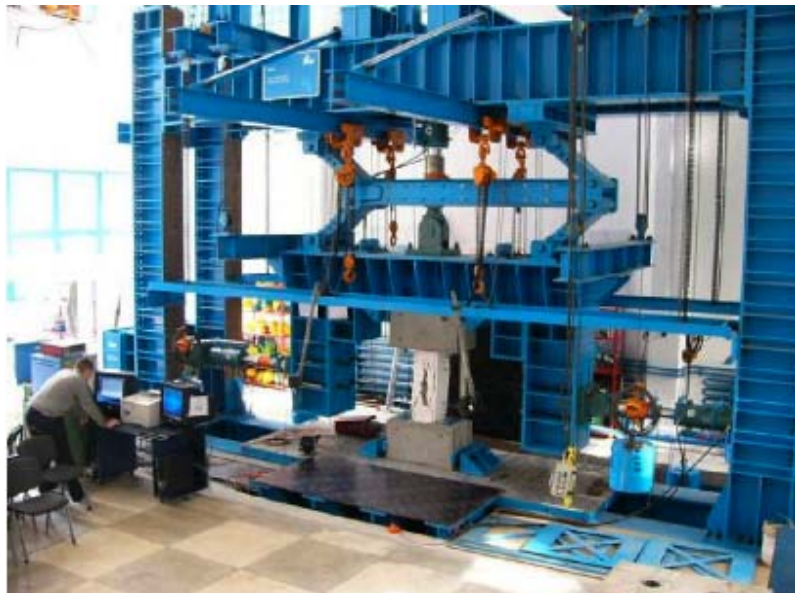
Figure 3. Reaction frame and Column Specimen
