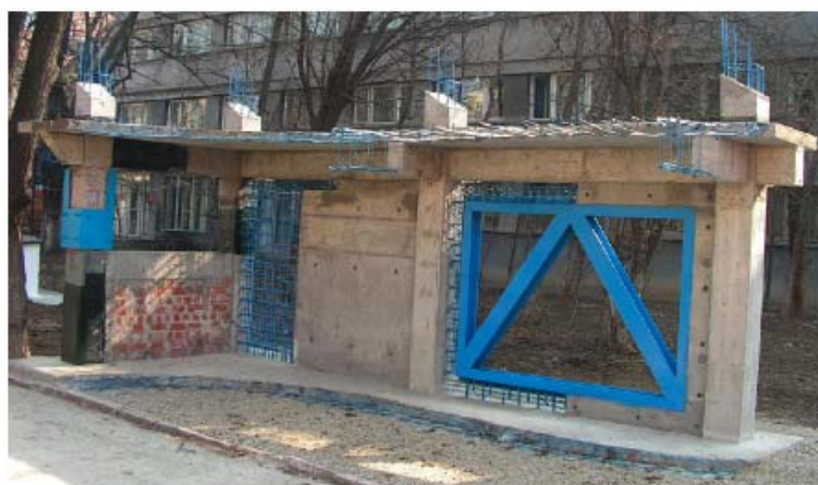
Figure 26. Model frame with retrofitting solutions
