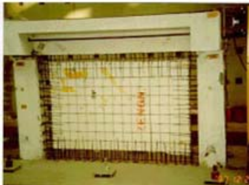
Figure 14. Strengthening of an epoxy repaired bare frame by 3D wire panel
