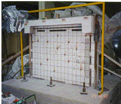
Figure 7. Integrated damaged infill wall and two sided wire mesh with shotcrete
