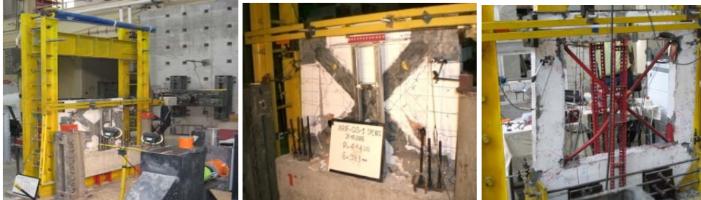
Figure 7. Pseudo-dynamic testing facility and the specimens
