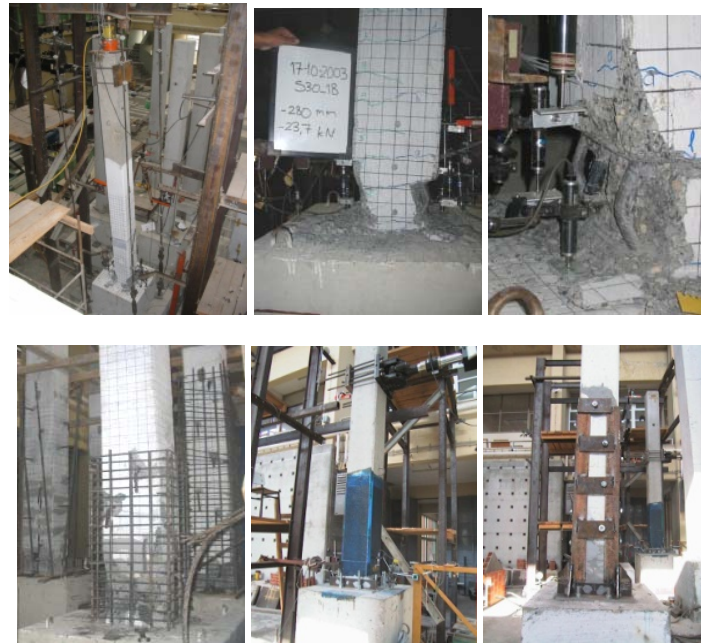
Figure 5. Full scale original and retrofitted column tests
