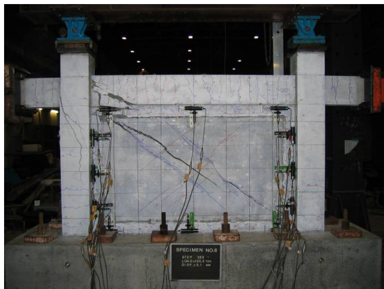
Figure 3. Example of seismic retrofitting experiment using UFC (Ultra High Strength Fiber Reinforced Concrete). The thickness of wall is half and the shear strength of wall is 1.5 than usual wall. (Fukuyama H., et al., 2009)
