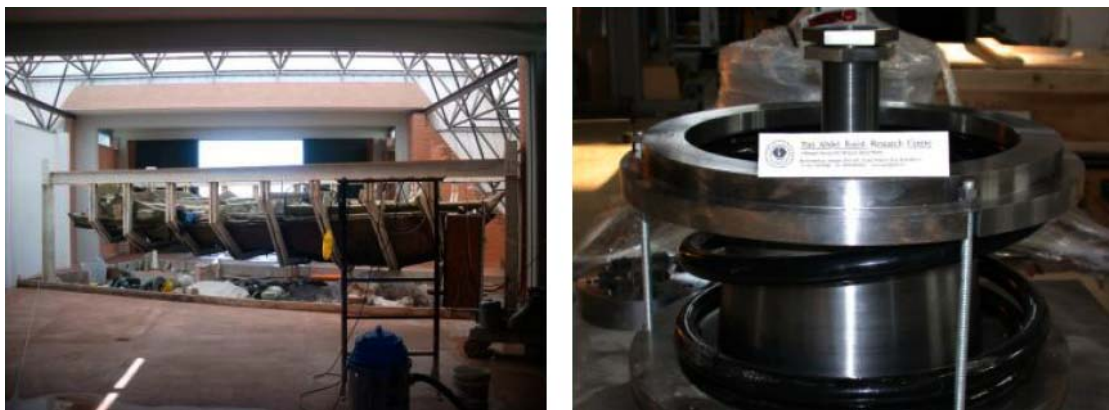
Figure 27. The wooden Roman ship excavated at Ercolano (Naples), in seismic zone 2, which was recently protected in the local museum by means of three-directional (3D) isolators formed by 3 spheres and a recentering rubber cylinder for the horizontal SI and a spring and a VD for the vertical one
