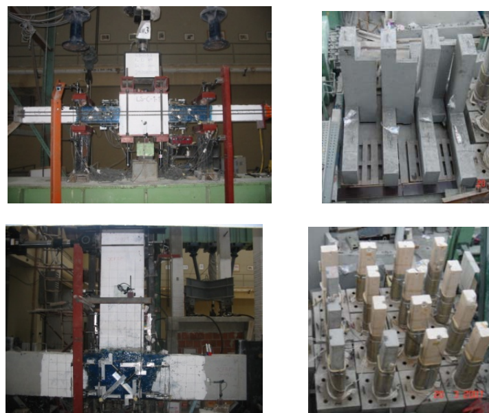
Figure 6. Column and beam-column joint specimens, and accelerated corrosion test specimens
