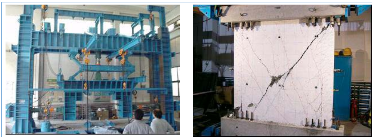
Figure 19. (a) Reaction frame donated by JICA, and (b) CNRRS tests on RC shear wall
