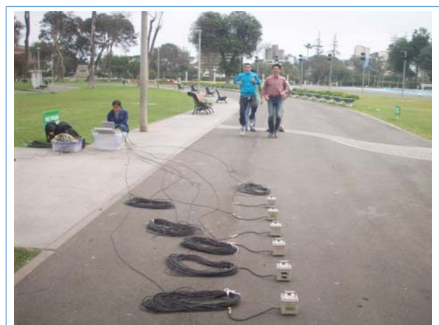
Figure 6 A linear arrangement setting a distance between sensors of 0.5–2.0 m in Reserva Park, Lima
