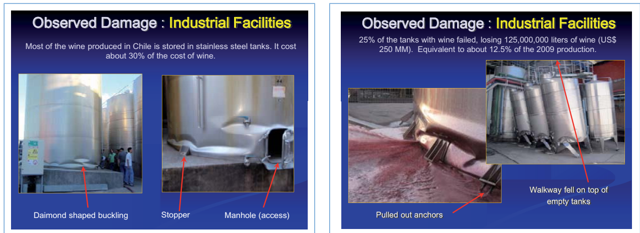
Figure 25 Failed stainless steel tanks and loss of wine
