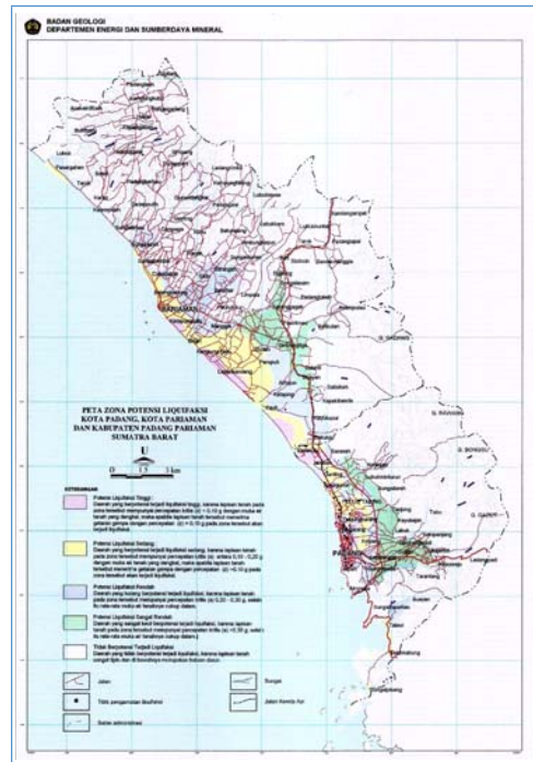
Figure 6 Liquefaction hazard map
