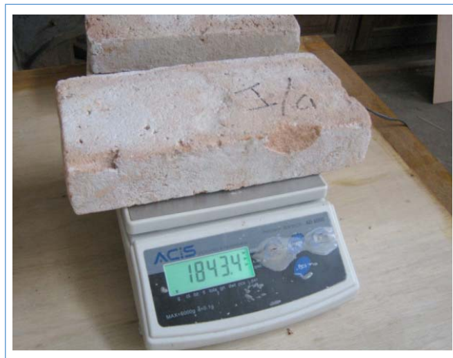
Figure 5 UNP Research Team Weighing Brick Sample
