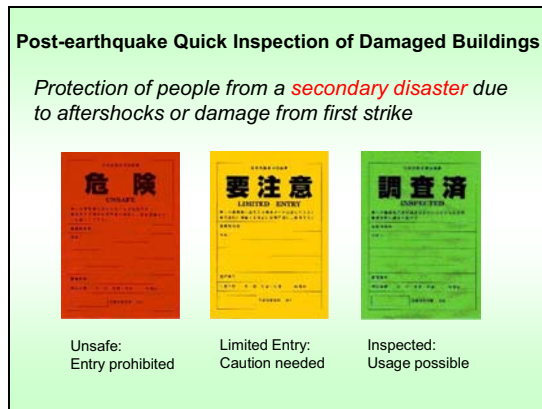
Figure 5. Post-earthquake quick inspection of Damaged buildings
