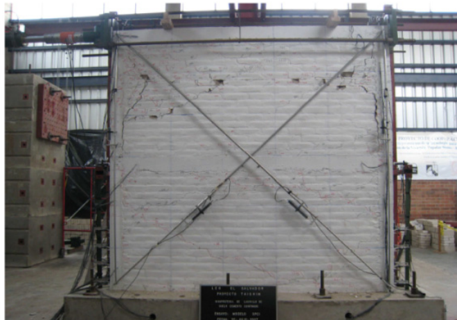
Figure 8. Test on confined masonry wall
