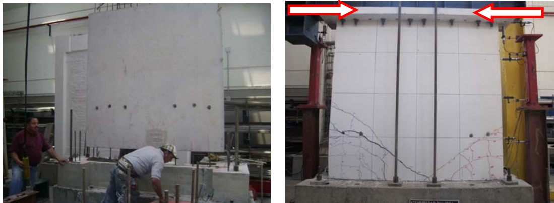
Figure 8. Reinforced concrete precast panel construction system for low cost housing has been tested at LSL of CENAPRED during the last year
