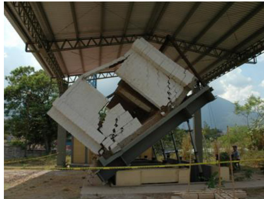
Figure 6. Tilting table system constructed in UES.
