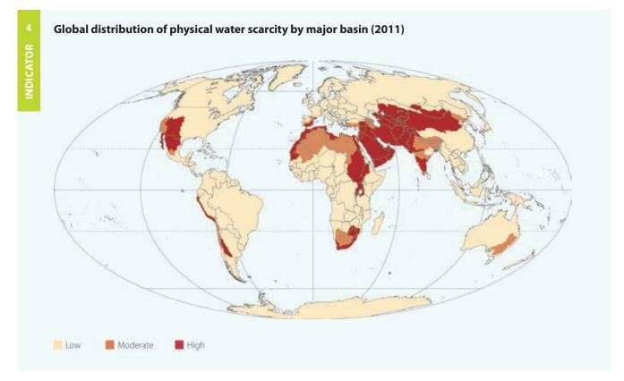
Note: The map shows the global distribution of water scarcity by major river basin based on consumptive use of water in irrigation. Source: FAO (2011, map 1.2, p. 29).
