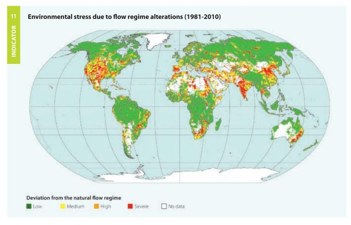
Note: Natural flow regimes are heavily modified by water abstractions and dam operations. The indicator "environmental water stress due to flow regime alterations" is used to assess the hydrological alterations resulting from these impacts (Schneider et al. 2013). Daily time series of modified and natural river discharge were simulated by the global water WaterGAP3 model on a global 5×5 arc minute grid (i.e. about 8×8km at the Equator) considering over 6 000 large dams.
