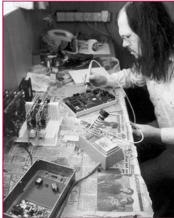
Soldering circuits for 20-watt FM transmitters in Brixham, UK.
