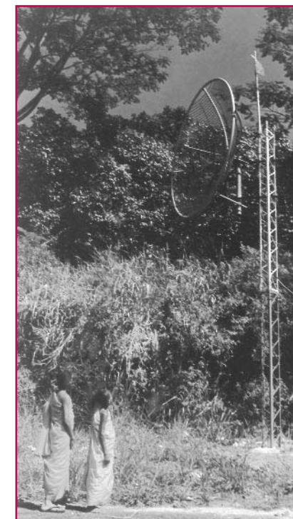
In Kothmale, Sri Lanka, the national government provided land, tower and antennas. These made it possible to set up microwave transception, telephone, twenty-four hour link to Internet and FM transmission.
