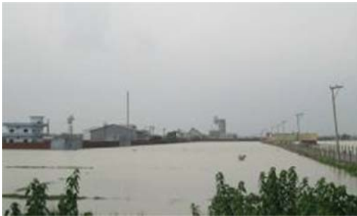
Photo 18: Factories in the Kamariya VDC and inundation nearby farmlands due to the removal of soil by factories and lack of proper drainage
