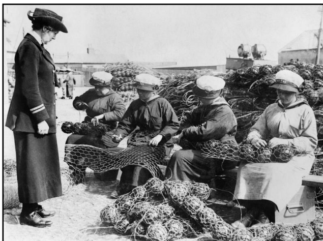
Figure 4. Ratings of the Women’s Royal Naval Service (WRNS) wiring together glass floats for an anti-submarine net, possibly in Lowestoft, under the supervision of a WRNS officer in 1918. © IWM (Q 19640)
