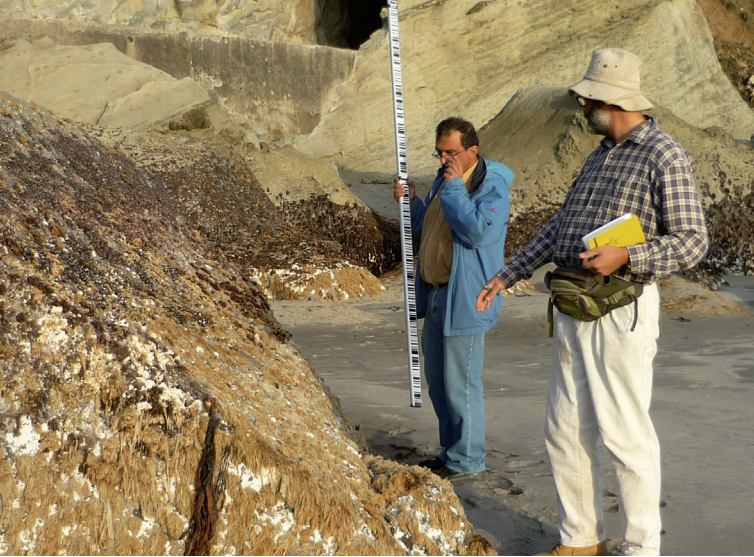
UNESCO experts measuring the change of height in the coastline after the earthquake, Bío Bío Region, Chile. © UNESCO Santiago.
