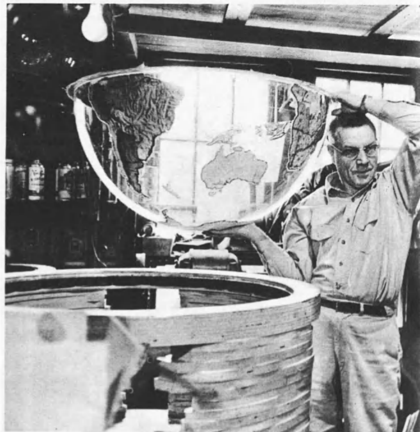
FLAT EARTH. Like a flash-back to an old historical belief, the earth is flat on this plastic sheet (left) but it will be heated, then inflated with air to achieve the rounded contours of our planet (above). These large globes for schools are painstakingly made by hand.
