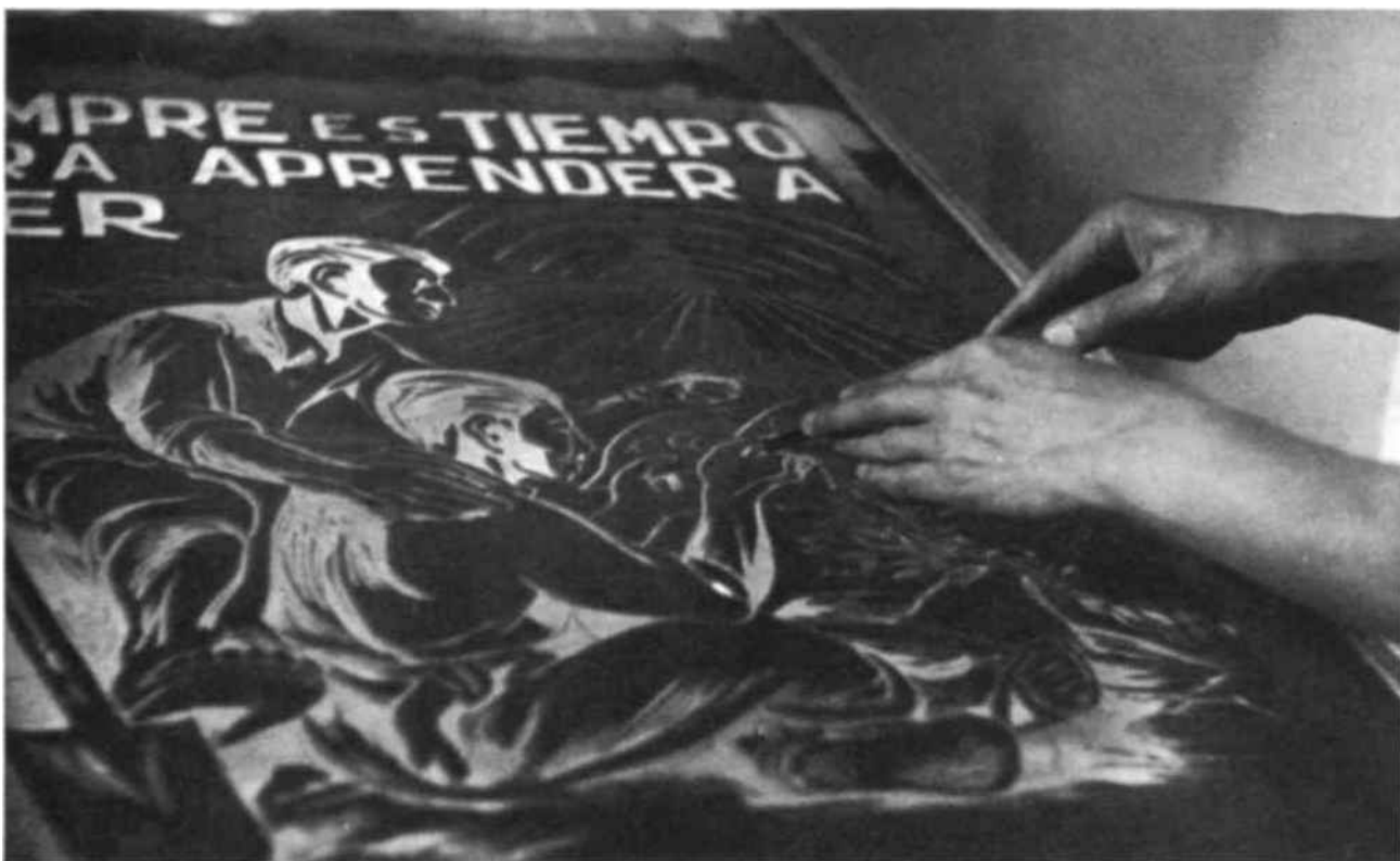
Artist engraves poster design directly in a mixture of paraffin wax and beeswax spread on glass plate. He cuts right down to glass (see diagrams on right) and can easily correct any mistakes by melting a candle over the wax plate.
