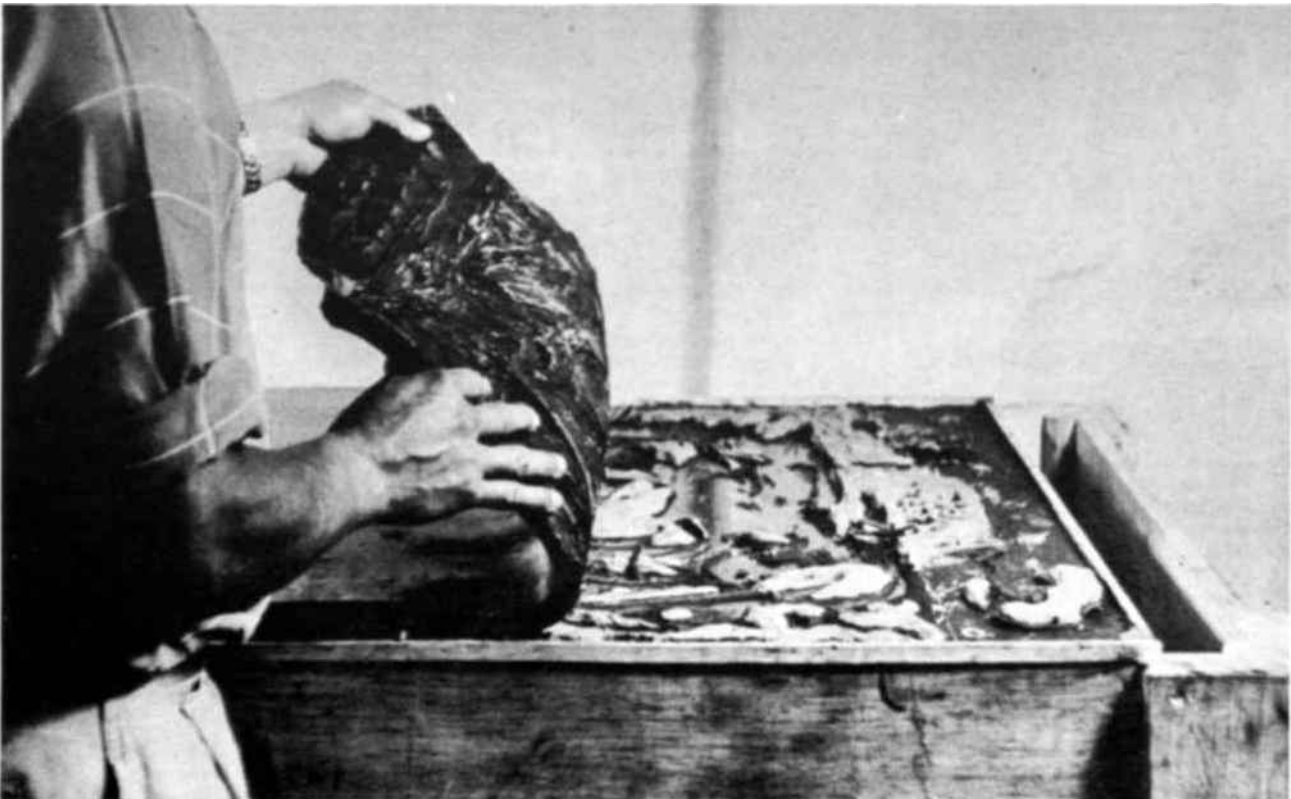
After engraving, a mixture of glue and glycerine is poured over wax. Finished plate (here being removed) has a rubbery texture. Poster can be printed from it by inking its surface, laying down a sheet of paper and smoothing it down by hand.
