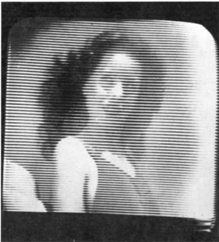
In this photo, the lines (formed by dots) which make up all television images have been greatly exaggerated to show how a picture is reproduced on the screen.
