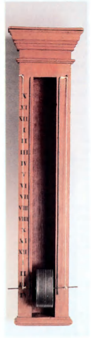
An early 19th-century French water clock or clepsydra. The water is contained in a drum divided by partitions pierced by small holes. It slowly flows through the holes, causing the drum to turn and descend between the graduated uprights as the 2 cords attached to its axis unroll.
