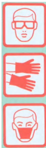
Pictographs showing items of protective clothing to be worn when handling chemical products. From top down: goggles, gloves, face mask.
