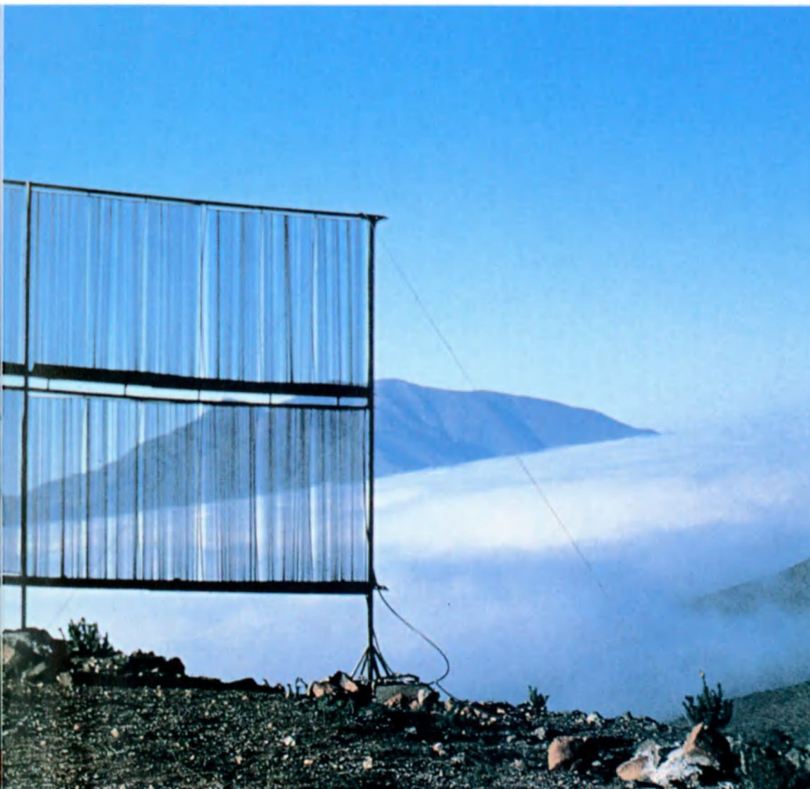
The strips in this screen serve to trap moisture from clouds and mist. The technique, developed in the Andes, is now also used in India and the Gulf region.
