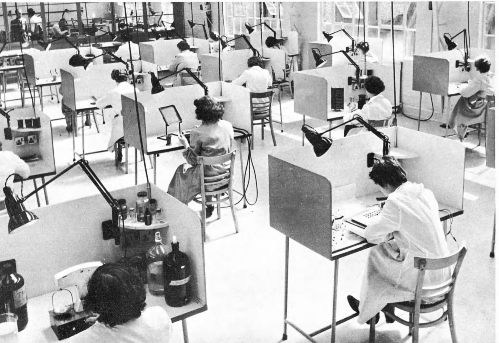
MAGNETIC MEMORY MAKERS. Electronic computers are progressively getting bigger and bigger in terms of work capacity—they can now average ten thousand operations a second—but the components are getting smaller and smaller. Today transistors no bigger than a grain of rice have replaced radio valves and some cells which store information are a 250th of a millionth of an inch in diameter. Below, magnetic "memory stores" for use in electronic digital computers being made in a British factory. Above, windings forming part of the "memory", into which information is fed and stored, are soldered into position. Wires are threaded through tiny cores, sometimes only one-twentieth of an inch in diameter, so threading the thousands that are used demands a keen eye and much dexterity. This wiring by hand illustrates the vital part still played by the skilled worker in the age of automation.
