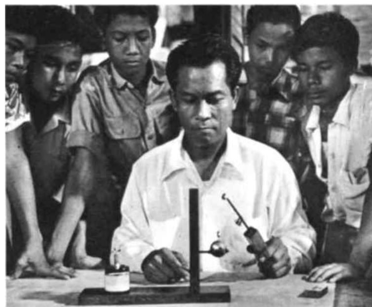
An old paste pot or an ink bottle can double as a laboratory burner with the help of shreds of cotton, a metal tube and some ingenuity. This Philippine teacher was one of the students who attended a training course conducted by Mr. Holbro.
