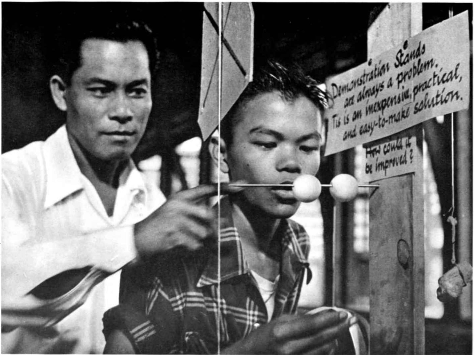
Why does an airplane fly? With two ping-pong balls and a knitting needle, a Philippine teacher demonstrates Bernoulli's principle. The pressure at the side of a stream of air is inwards toward the centre of the stream. Pupils can prove this to their own satisfaction; when they blow on the balls, these come together.
