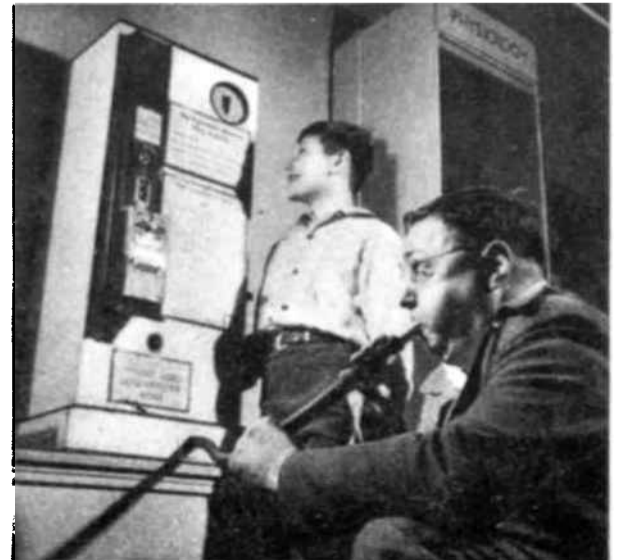
"Going up". While father blows hard into the tube, his son watches the needle rising on the Vitalometer, an instrument in the Cleveland Health Museum which measures lung capacity.
