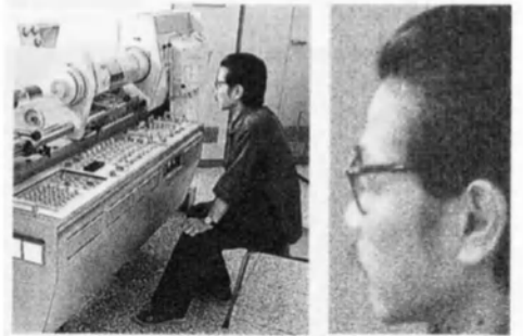
28. Electronic scanners (right) can be used to process images for printing. The image is fitted onto a revolving drum and reproduced by the scanner as a pattern of tiny dots. Far right, halftone dots enlarged
