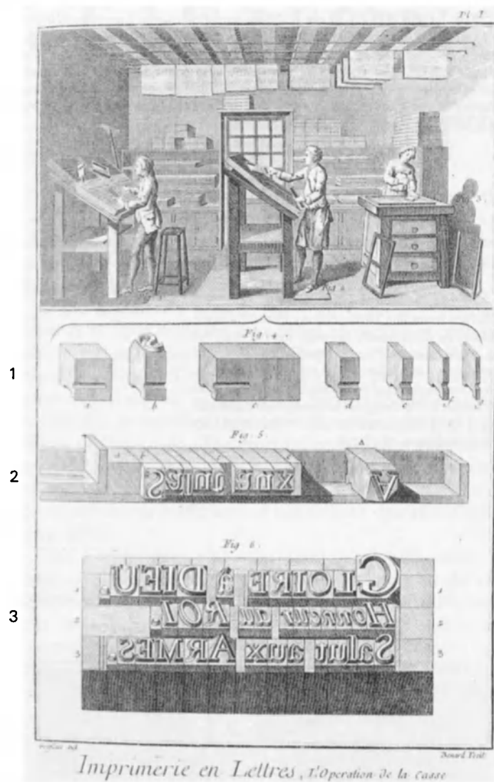
Plate from the Encyclopédie showing operations in the composing room of a printing shop. Top left, a compositor transfers metal type (such as the letter “S” and the different-sized blank spaces for separating words shown in 1) from typecase to composing stick (2) to make a line. Top centre, another compositor moves a line to a tray or “galley” of type where, with other lines (3) it forms part of a page. Top right, a third compositor has locked two pages of type inside a metal frame and is levelling the printing surface ready for the press.
