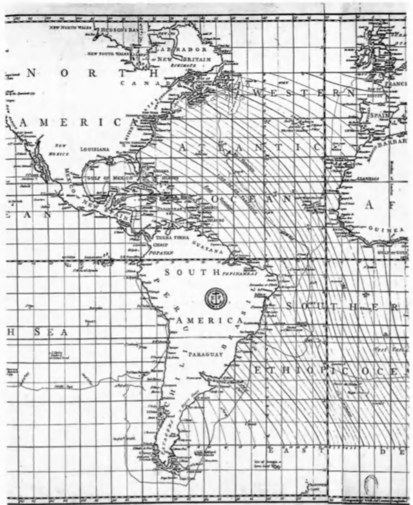
Chart of magnetic variation was drawn by the English astronomer Edmond Halley in 1700 and corrected in 1756 by William Mountaine and James Dodson.
