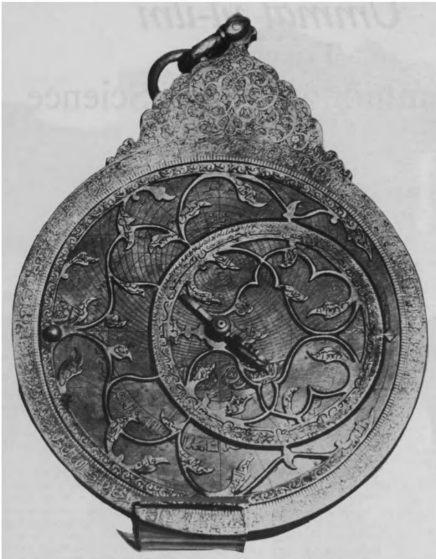
Left, Persian brass astrolabe dating from the XI/17th century. Astrolabes were used in computing the position of the stars and the movement of the planets, as a means of telling time, and as navigational instruments. They date back to before Islam, but were vastly improved by Muslim astronomers. Right, diagram from an Arabic manuscript, dated 602 AH/1205 AD and now in the Topkapi Museum, Istanbul, which explains the working of the astrolabe.
