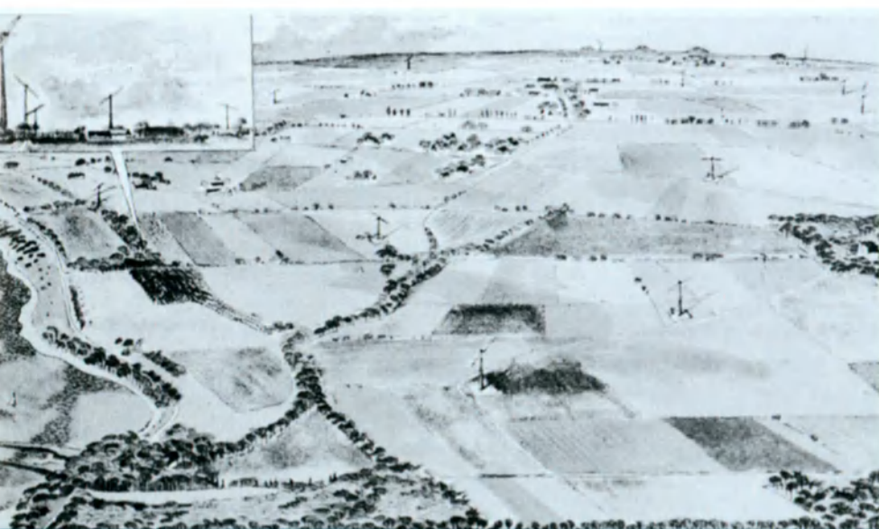
Left: "Solar Sweden" in 2015. Wind power development with a station of 4 MW wind turbines. Height about 100 metres, blade length 80 metres. The configuration follows guidelines for location proposed by the National Board for Energy Source Development. Cables are laid underground, but this would not be the case in less favourable soil conditions.
