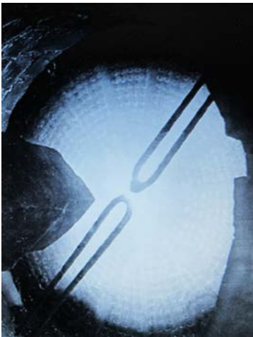
The electric arc under magnetic influence in the chamber inside a Birkeland-Eyde furnace.
