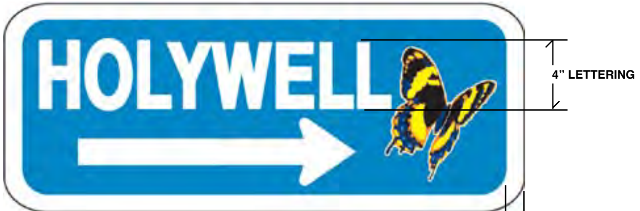
Fig. 35. 30"x 12" Directional Sign specifications
