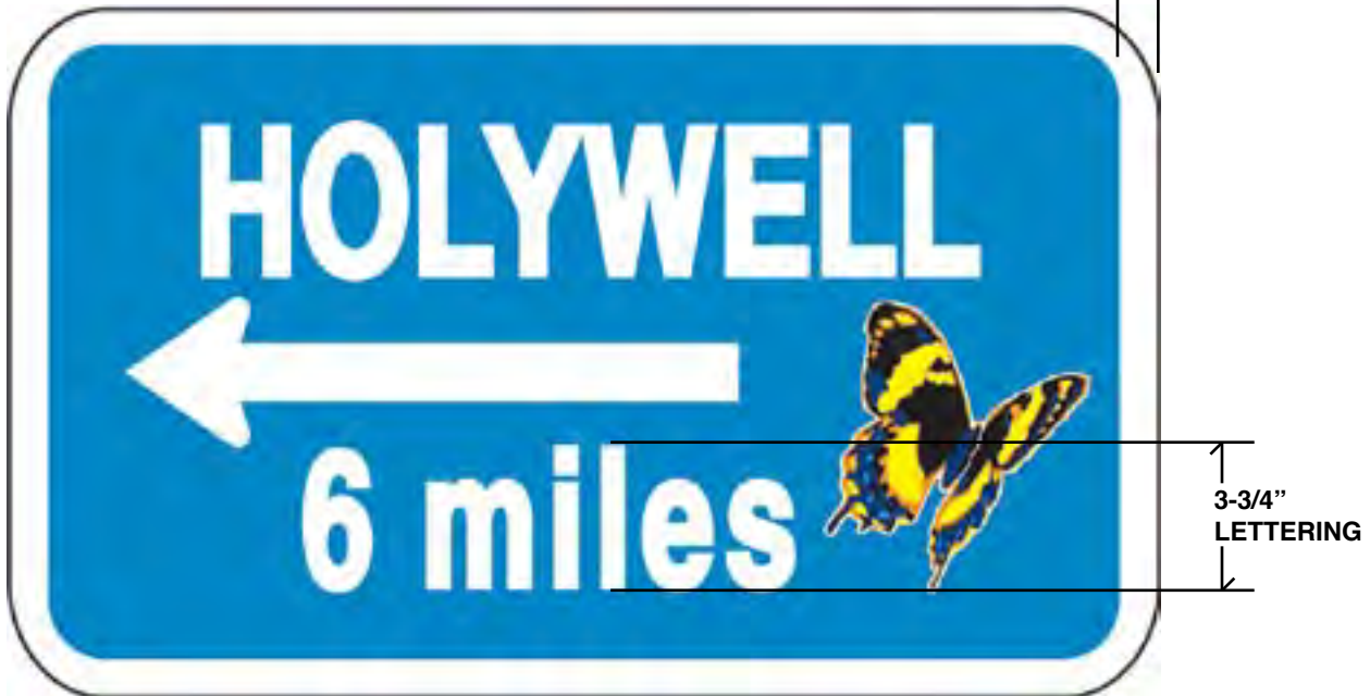
Fig. 36. 30"x 18" Directional Sign with mile indication specifications
