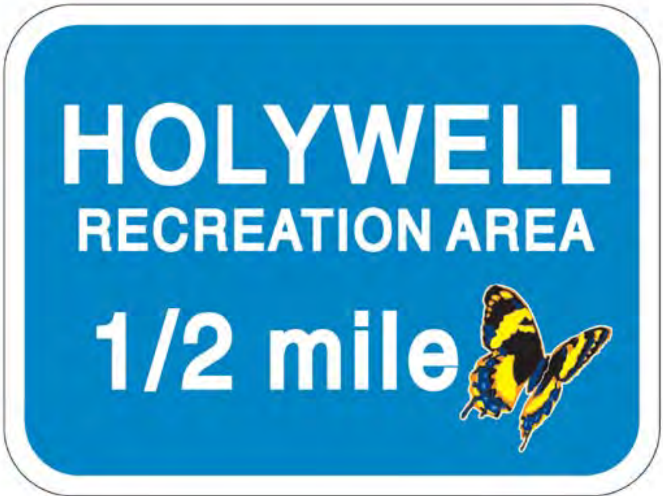
Fig. 39. 48" x 36" Approach sign with mile indication to be placed 1/2 mile before Holywell destination
