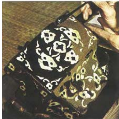
5. Fixing the powders When the lacquer has dried, paint another layer of lacquer to fix the gold.
