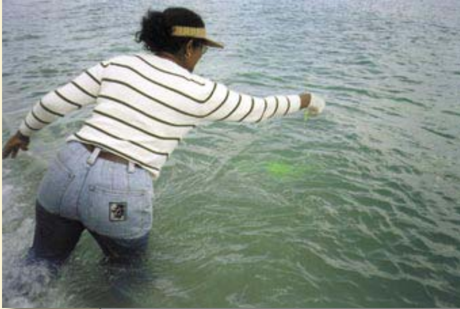
Measuring longshore currents with fluorescent dye, St Lucia, 2001.
