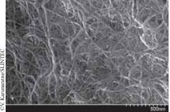
Carbon nanotubes produced bv Prof Verania Karunaratne at the Sri Lanka Institute of Nanotechnology using Sri Lankan Vein graphite. a type of rock which can contain up to 99% carbon. Plants exposed to carbon nanotubes grow better than usual, making nanotubes a promising ingredient for agricultural fertilizers.
