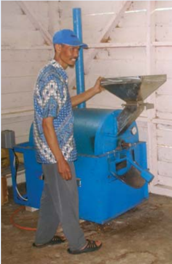
ABOVE The coffee milling machines in E3i village using electricity generated from micro hydro power. (c) UNESCO Jakarta
