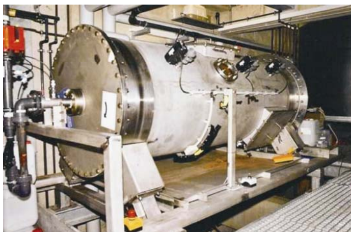
Figure 10 Pilot-scale Roto Bio Reactor, length: 4 m, diameter: 1 m, number of rotations: 4/h, quantity of PCL: 302 L/chamber, flow rate: 300 – 1000 L/h
