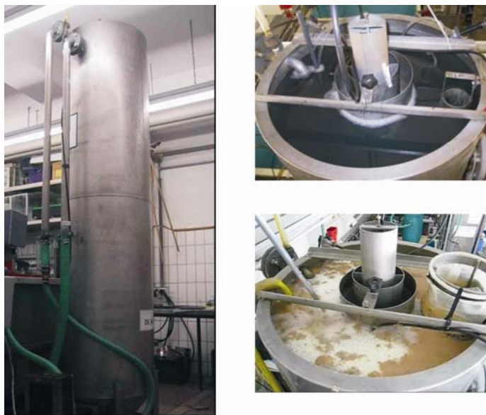
Figure 11 Dyna-PCL reactor (left). Empty Volume: 805 L, Mass of PCL: 350 kg. Flow rate: 350 L/h. Top view (right, top), formation of gas bubbles during denitrification (right, bottom).
