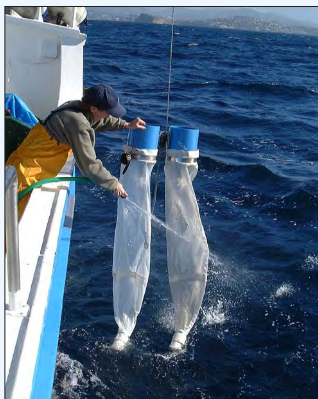
Plankton sampling using a Bongo Net.
