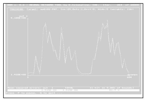
Fig.4 presents the output of the ANN (trained on 1981-82 data) fed by the 1983 input data, which is compared to the actual water levels for 1983 given by MIKE-11. This demonstrates the predicting capabilities of ANN.
