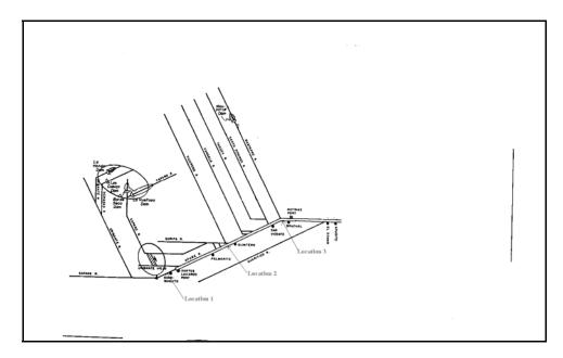
(Venezuela). The schematization of the river system is presented on Fig. 1. In this basin, one reservoir (*La Honda*) is in operation, one (*Las Cuevas*) is scheduled, and one (*La Vueltosa*) is under construction. In the near future, three reservoirs will be in joint operation, and this is the scenario that was considered.
