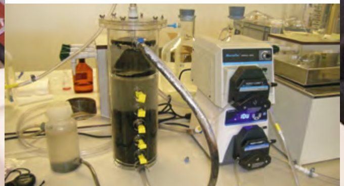
Lab-scale UASB reactor to treat olive mill wastewater.
