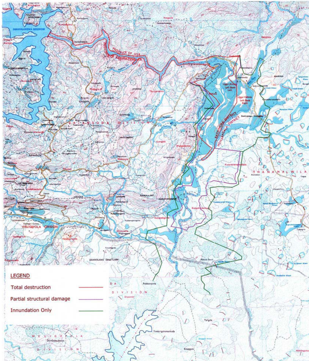
Figure 4.18 Inundation areas in the Walawe basin in the event of a Samanalawewa dam break Source: Talagala, 2008.
