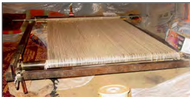
Fig., 17 Metal horizontal loom; in metal loom, warps are wrapped around a rod called Fandak (instead of Sardār )
